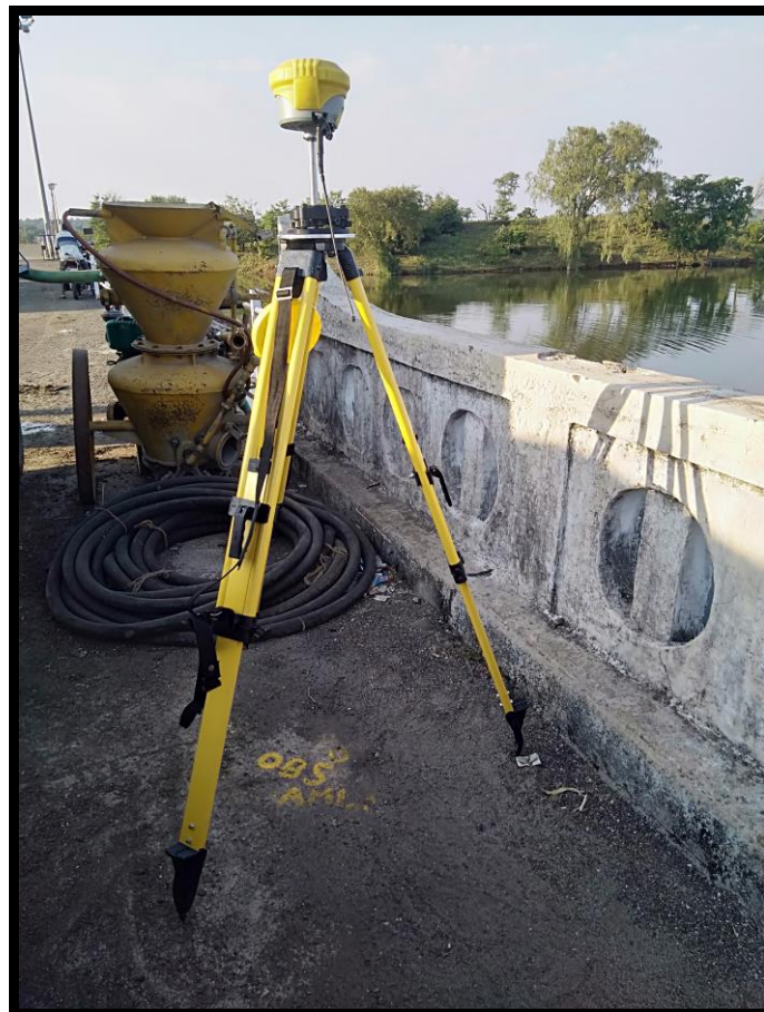
RTK Base Set up At Dam
